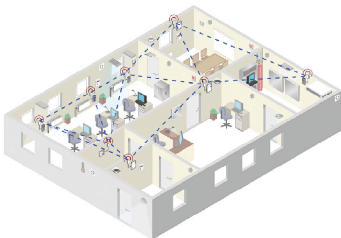
A mesh network installation
